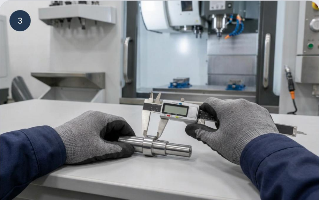
Machining · shaft inspection with a digital caliper
